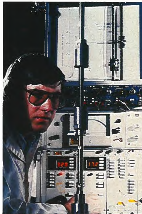
Acoustic emission monitoring of tensile test.
