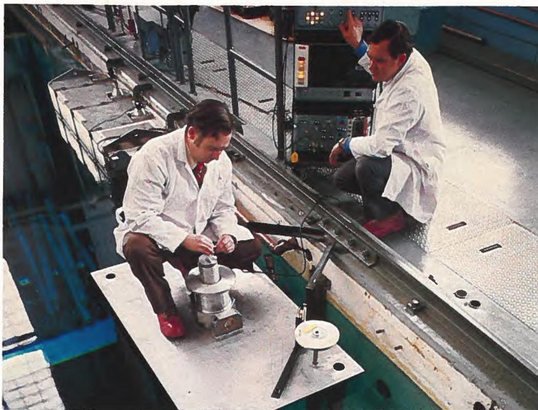
In large measure the excellent safety record of the CANDU reactor is due to the development of equipment capable of testing the systems safeguards. One such example is shown above testing the spent fuel safeguard system. It was developed by the Chalk River Nuclear Laboratories.
