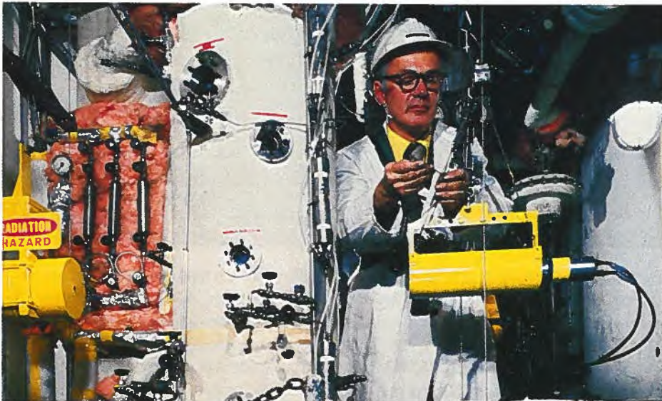
Radiographic instrumentation for flow visualization in heavy water towers.
