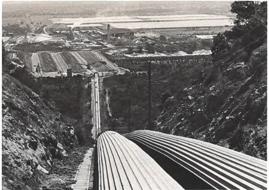
Twin covered conveyors carry bauxite ore the Darling Range in Western Australia to an Alcoa alumina refinery.
