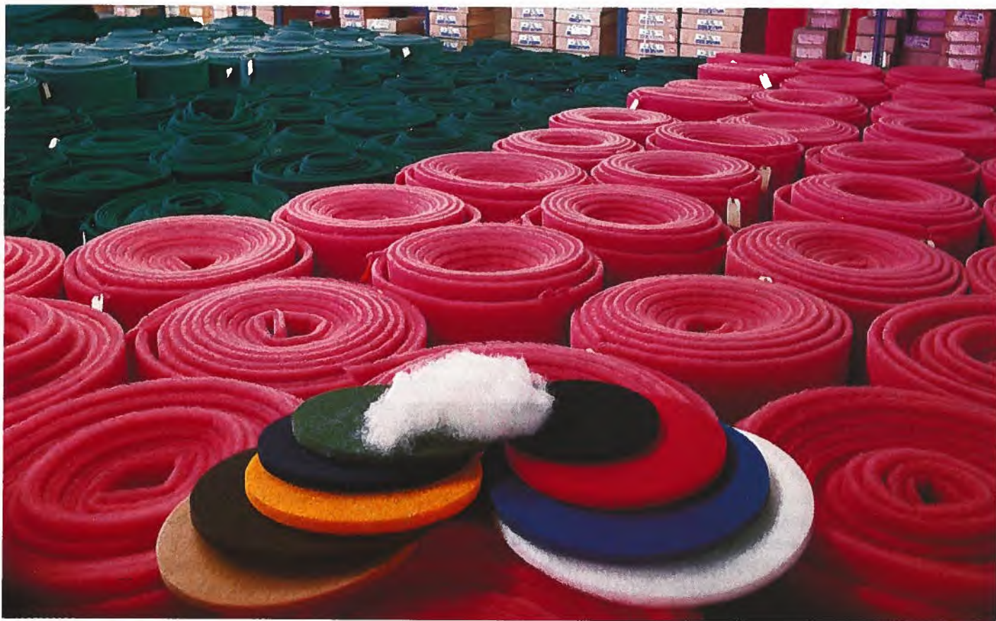
Rolls of polyester and nylon cleaning pad material await shipment to overseas markets in Empro's warehouse at Bramalea, Ontario. Customers in 20 countries cut floor maintenance pads to their own specifications from the rolls. Empro also ships fully manufactured pads oversea in palletized bundles as seen in the background.
