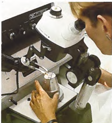
Bell-Northern technical staff wires a laser (about the size of a speck of black pepper) into a fibre optic communications system.
