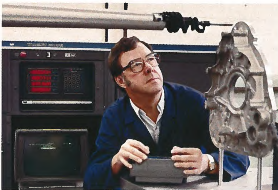
The dimensional inspection of light-alloy castings has been reduced from 300 to 40 man hours by employing high technology equipment. Microelectronics allow all measuring operations to be pre-programmed in this 5-axis manipulator.
