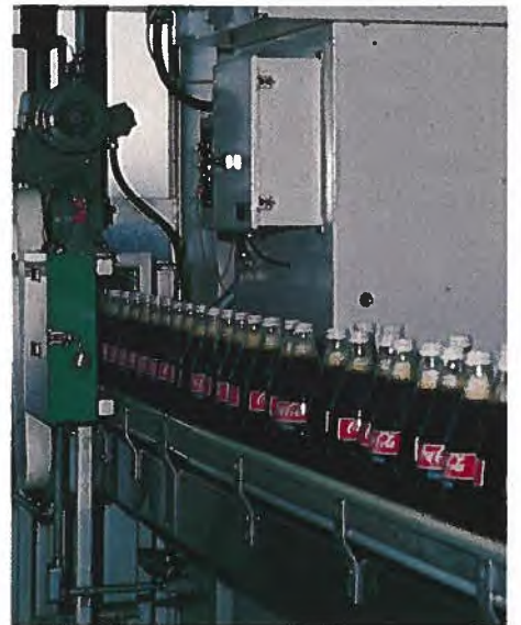
The LaserMark system being used to mark the caps of Coca-Cola bottles.
