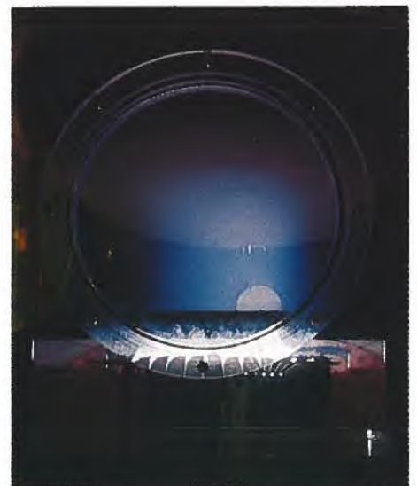
The discharge cavity of a large high-energy laser.
