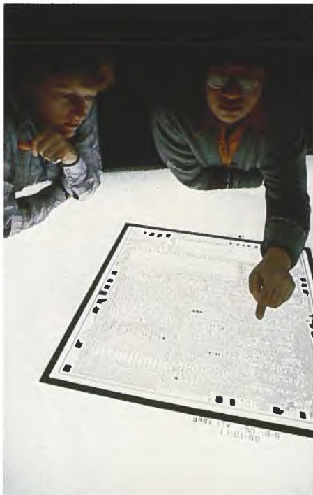
Canadian design engineers check the plot of an electronic circuit prior to mask making.
