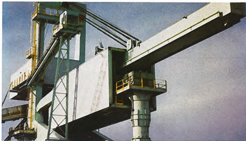
This 8 000-ton per hour coal shiploader designed and built by Dominion Bridge-Sulzer (DB-S) is in operation at Thunder Bay, Ontario.
