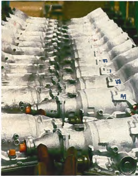
Vehicle transmissions roll off a Canadian automotive plant assembly line.
