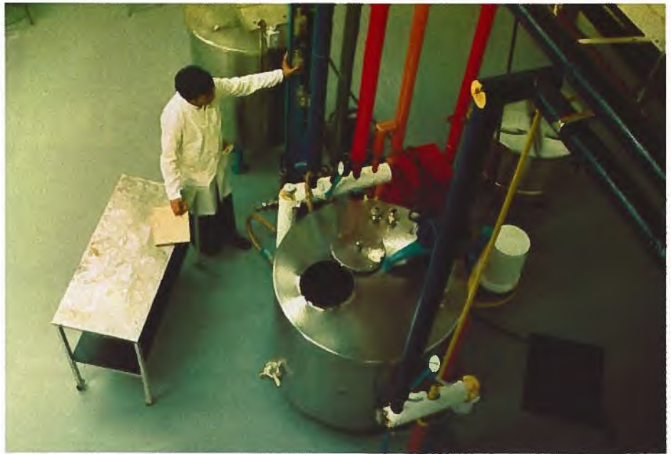
Enzymes used in Diagnostic Chemicals' diagnostic kits are extracted in this enzyme reactor.
