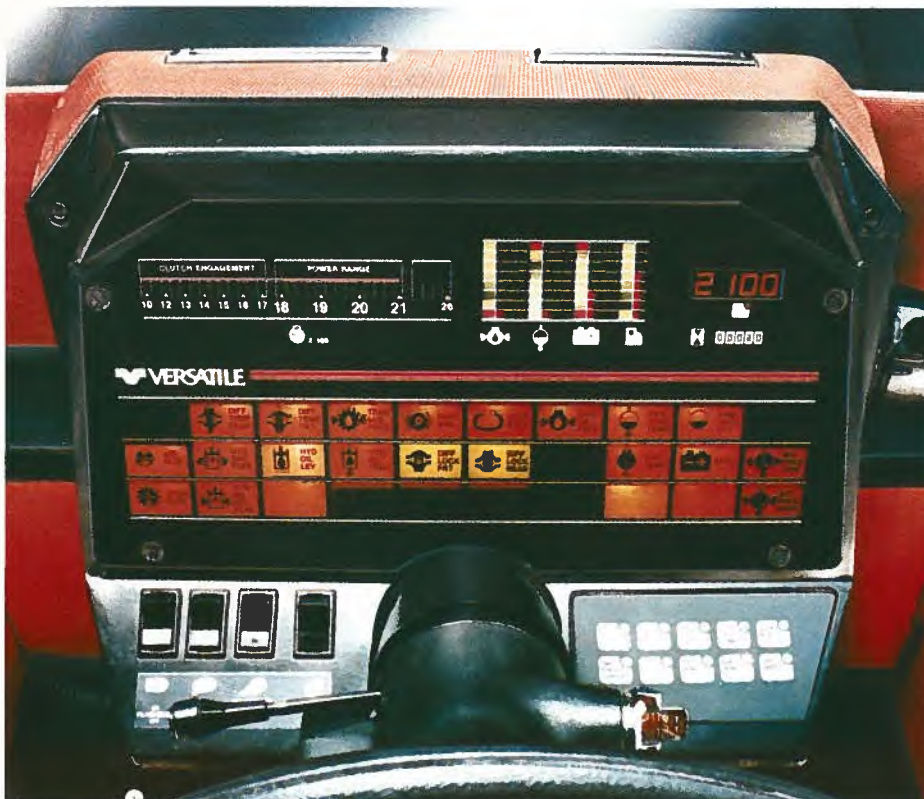
The dashboard of the Versatile 1150 tractor has an improved automated sensing and reporting system which enables the driver to keep an eye on the main operations.
