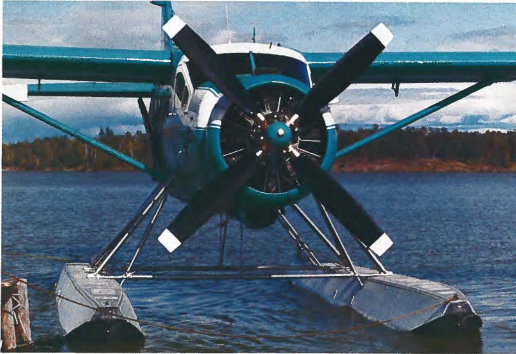
A de Havilland Otter re-engined by Airtech with a PZL 1 000 h.p. engine and four-blade propeller.
