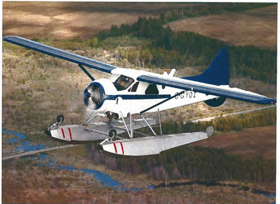
With new PZL 600 h.p. engine from Airtech and floats by Bristol Aerospace of Winnipeg, this Beaver is back in business.
