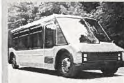
Over 20 — New Small, Heavy Duty Van Over 20 is a new small, low floor, highly accessible, heavy-duty truck not designed by Chrysler but based on the design of Mercedes-Benz. Designed for area transit operators and transit authorities. To achieve its very low, ground clearance, the van has been designed with the push-button advantage in its rear, allowing it to be raised or lowered. Its unique design allows it to be disassembled in an hour which includes the engine, transmission, front and rear axles, suspension and steering. The whole vehicle can be removed in less than an hour and returned to the same spot in time.
