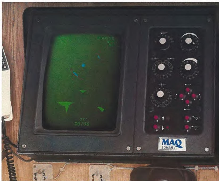
Scannar's MAQ commercial fishing sonar in place.
