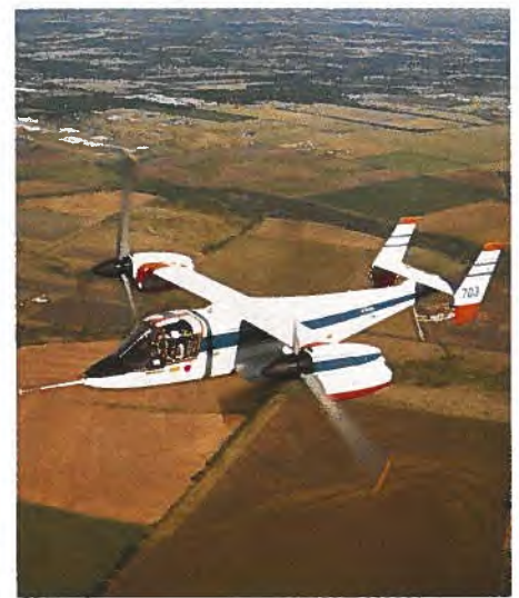
Tiit the engines and this Bell soars vertically.
