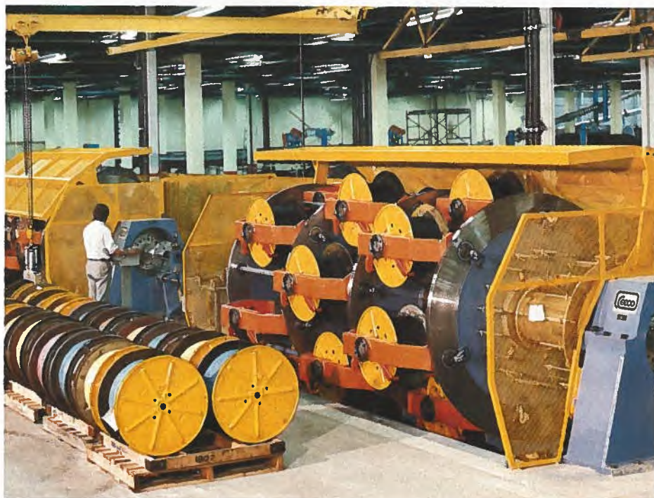
Planetary strander/cabler designed to accommodate 30, 30" bobbins
