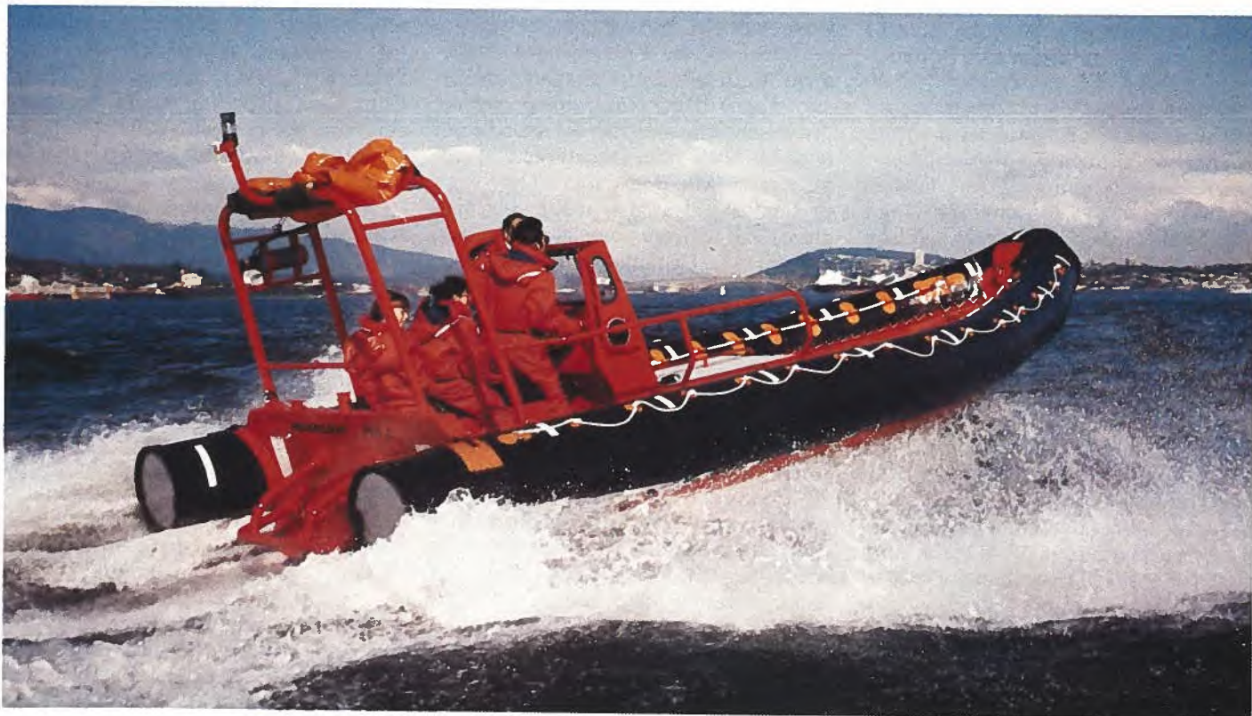
Twin-engine inflatable search and rescue boat.
