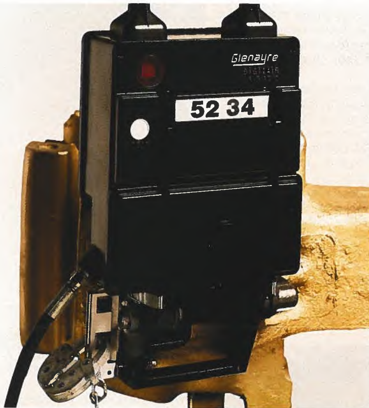
DIGITAIR (rear-of-train) monitoring system.
