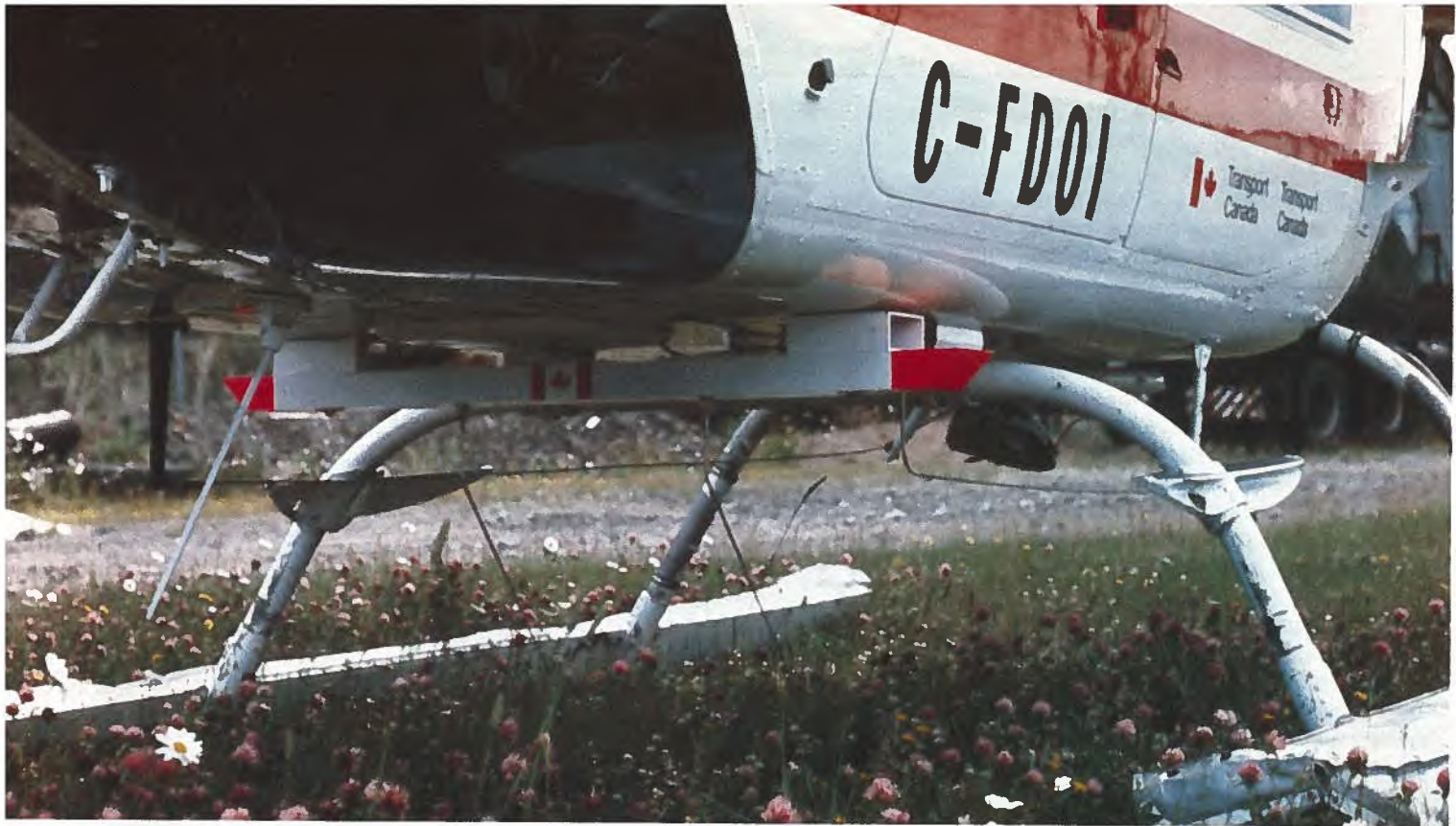
Helicopter antenna, the white bar across the aircraft's bottom.
