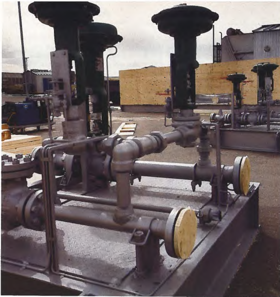
Enerflex-designed and produced gas compressor station for New Zealand shown being broken down into modules and packaged for shipping.
