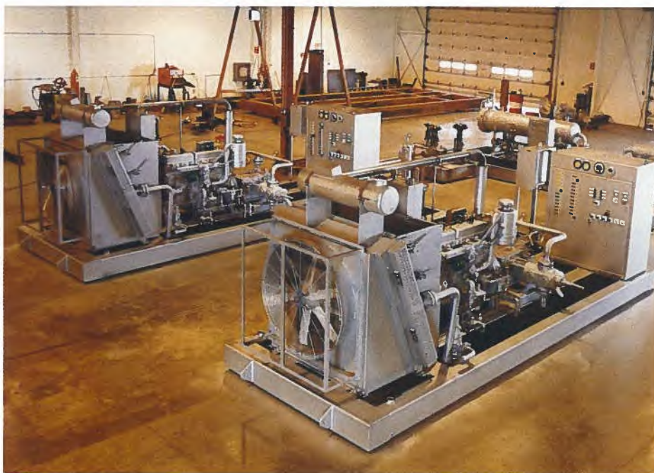
Overall view of compressor station assembled for testing in Enerflex's Calgary shop.
