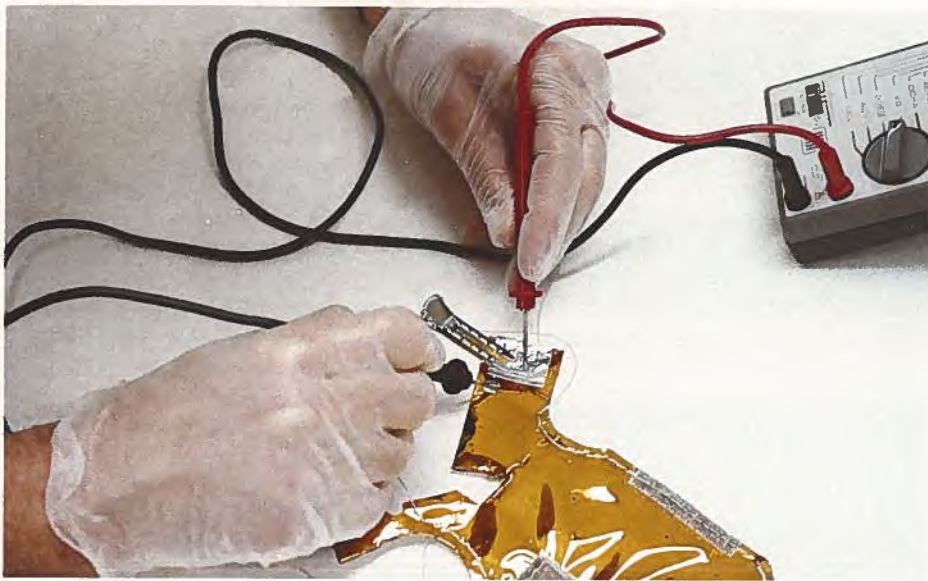
Resistance check of the five layers of thermal insulation which protect vital parts of the Olympus satellite.
