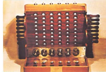
Wilhelm Schickard's Calculating Clock could multiply and divide as well as add and subtract.
