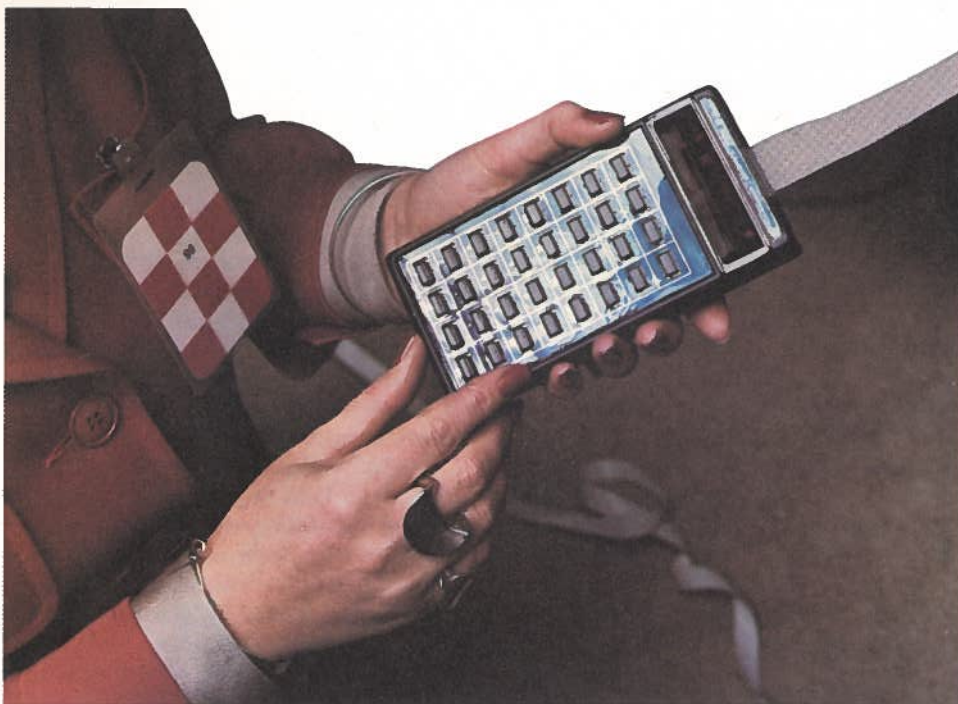
Keypad used for calling up "pages" of information for display on TV.
