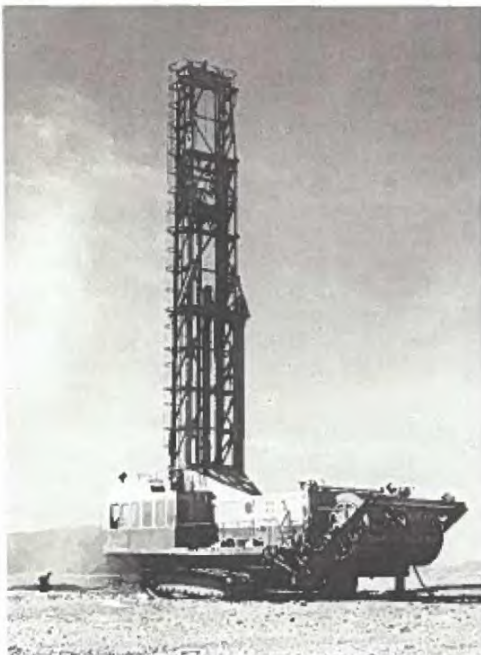
A huge Bucyrus-Erie churn drill at work at Gaspé Cooper Mines, Ltd., Murdochville, Quebec. Photo: George Hunter
