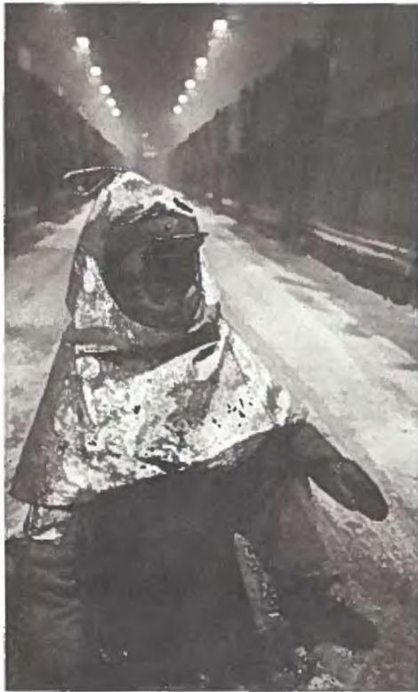
A worker wearing special safety clothing hand pokes the crust of an aluminium reduction cell (Soderberg pot) at the Alcan Aluminium Ltd. works in Arvida, Quebec. Photo: Alcan
