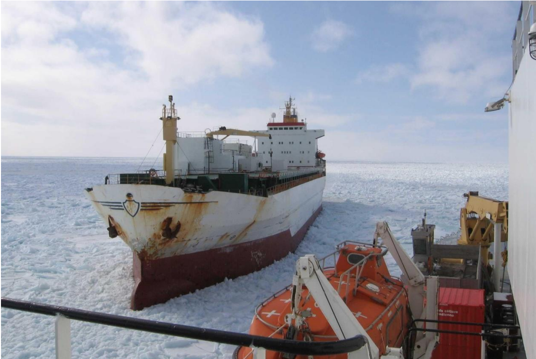
Figure 47 - Icebreaker backing alongside vessel to free it from the ice (CCG)
