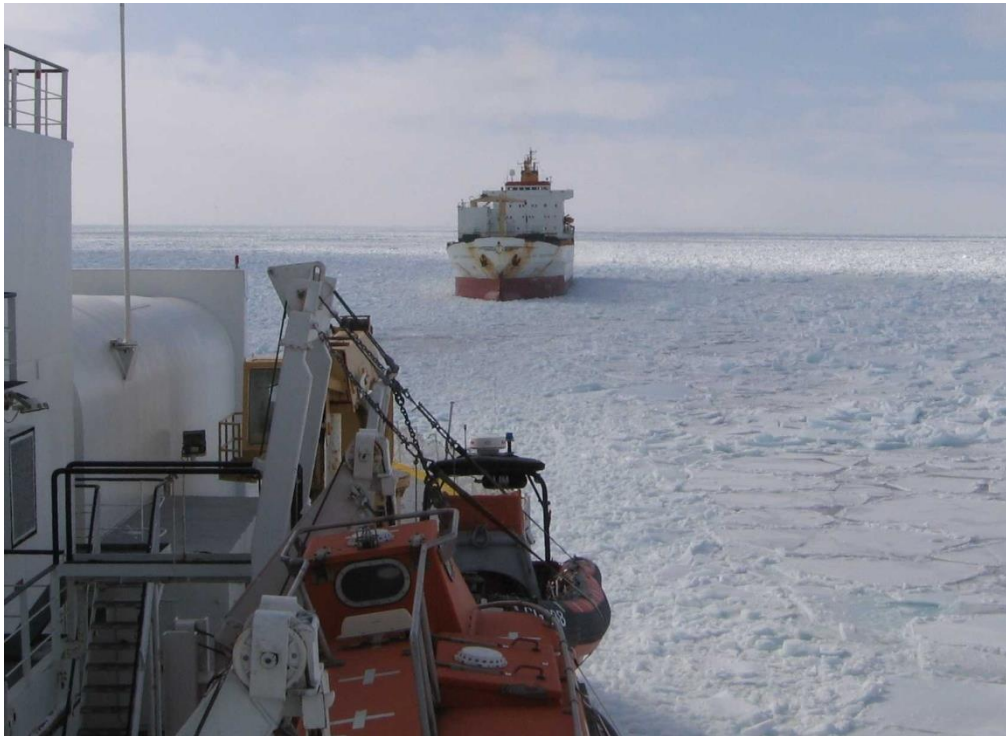
Figure 46 - The commanding officer of the icebreaker will determine a safe escort distance (CCG)
