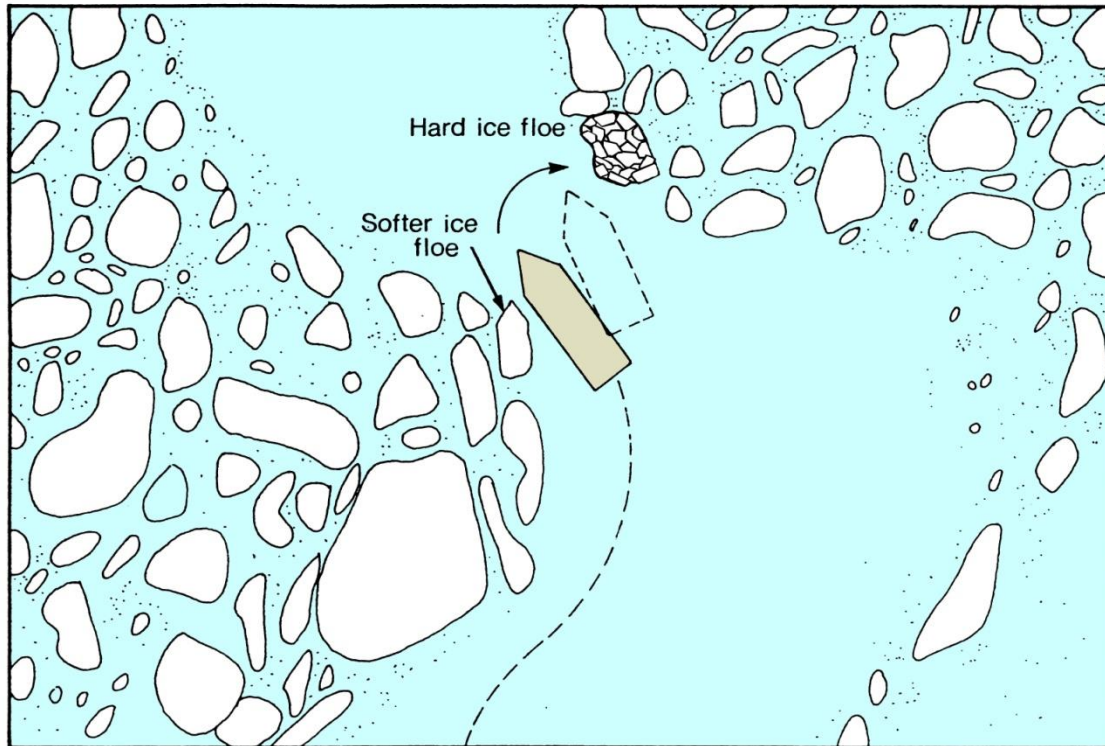
Figure 50 - Danger in turning in an ice channel (Courtesy of Capt. George Q. Parnell “Ice Seamanship”)
