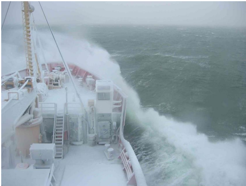
Figure 43 - Severe icing conditions (CCG)
