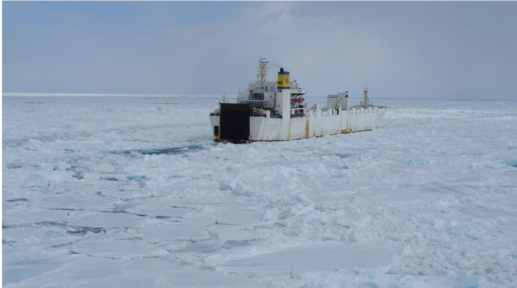
Figure 53 - Ice under pressure will close the track behind the vessel (CCG)
