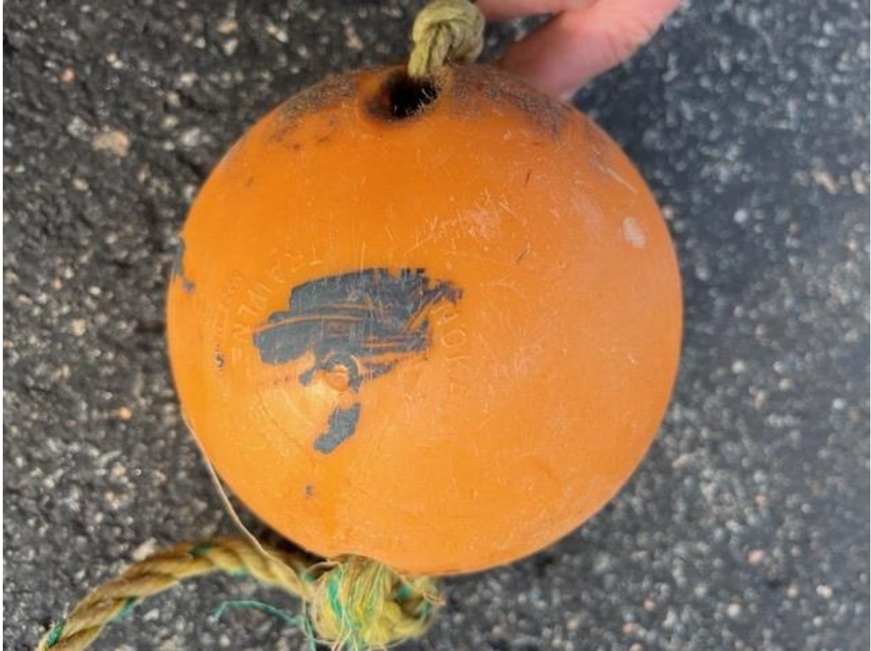
Fig. 3. Orange spherical buoy (diameter 5 inch; 12.7 cm) made of hard plastic. There are recesses located on opposite ends of the buoy through which 3/8 inch rope was passed as a means of attachment. The name and country of the manufacturer are visible (Nokalon, Denmark). The buoy had a crack in it. Photo credit: Ed Trippel, DFO.
