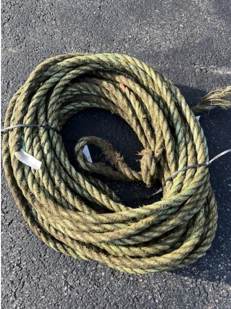
Fig. 4. Segment 1: 95 ft (29 m) of 5/8 in. float rope with a yellow tracer that included a DFO coloured buoy line mark. Photo credit: Ed Trippel, DFO.
