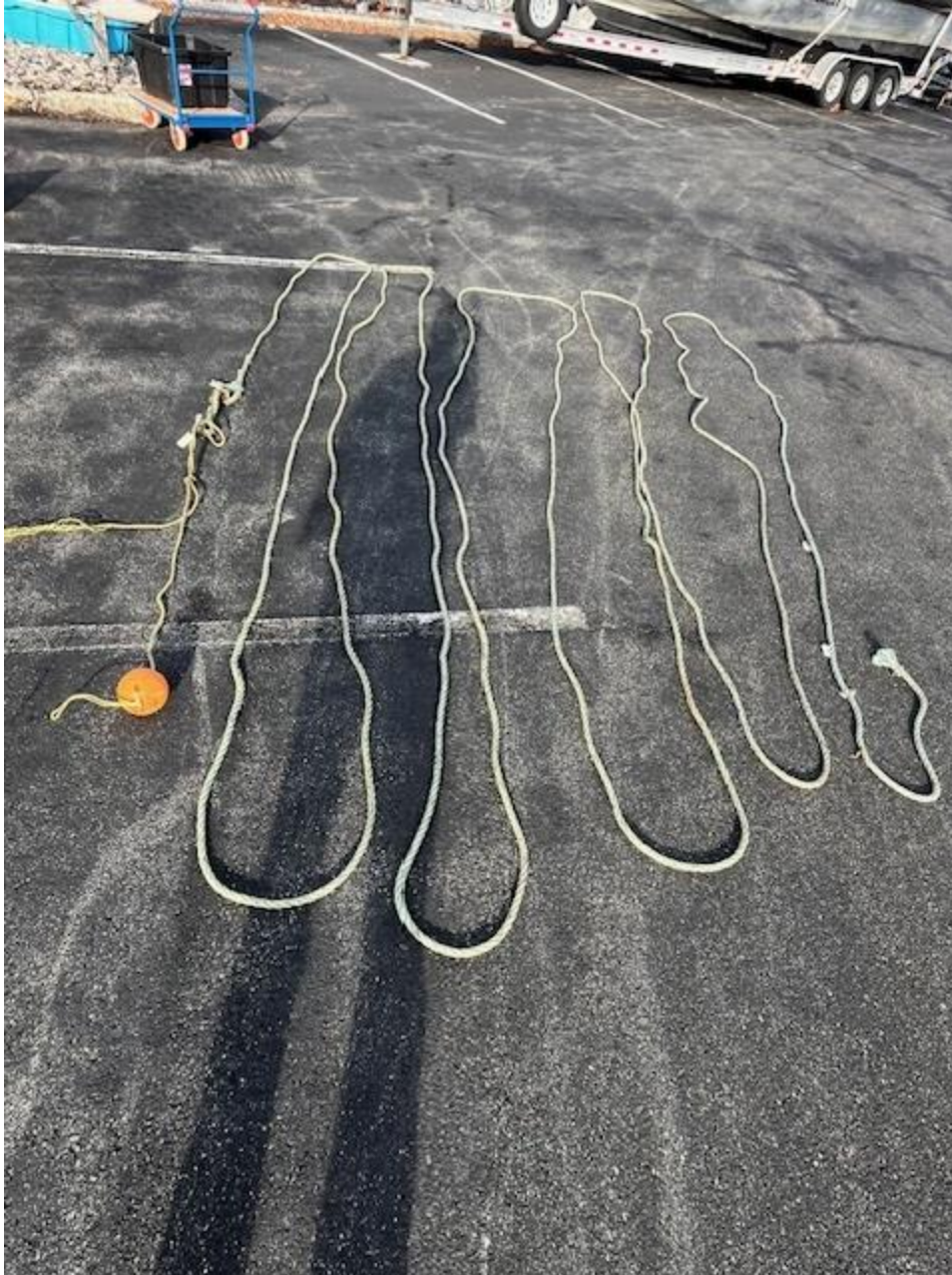
Fig. 6. Segment 2: 138 ft (42 m) of 5/8 in. sink rope with the remnants of the surface buoy system. 3/8 inch yellow polypropylene rope with green tracer was attached to an orange 5 in. (12.7 cm) diameter hard plastic buoy. A DFO coloured buoy line mark was present on the 5/8 in. rope. Photo credit: Ed Trippel, DFO.
