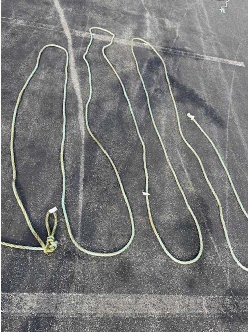
Fig. 10. Segment 3: 69 ft (21 m) of 5/8 inch float rope with a telemetry loop placed on December 3, 2025, this segment of rope included a coloured buoy line mark. Photo credit: Ed Trippel, DFO.
