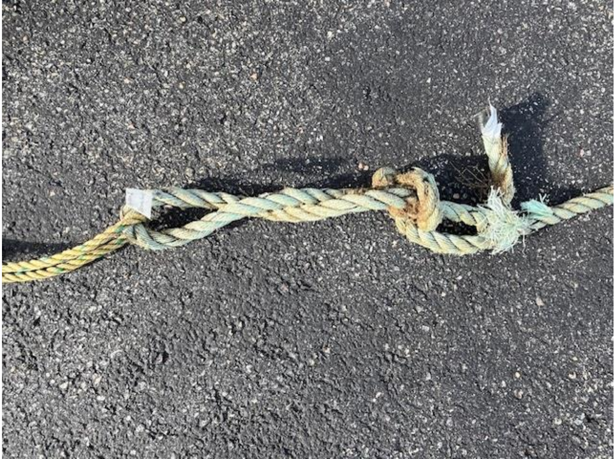
Fig. 9. Segment 2: Knotted loop of the 5/8 in. sink rope (with black tracer) to which the 3/8 in. Yellow polypropylene rope (with green tracer) was attached. Photo credit: Ed Trippel, DFO.
