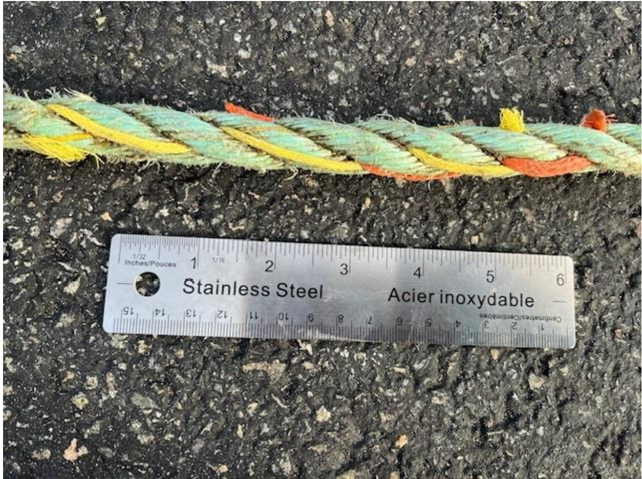
Fig. 14. Segment 3: Orange and yellow braided twines interlaced along a 7.1 inch (18 cm) section of 5/8 inch floating rope. Photo credit: Ed Trippel, DFO.
