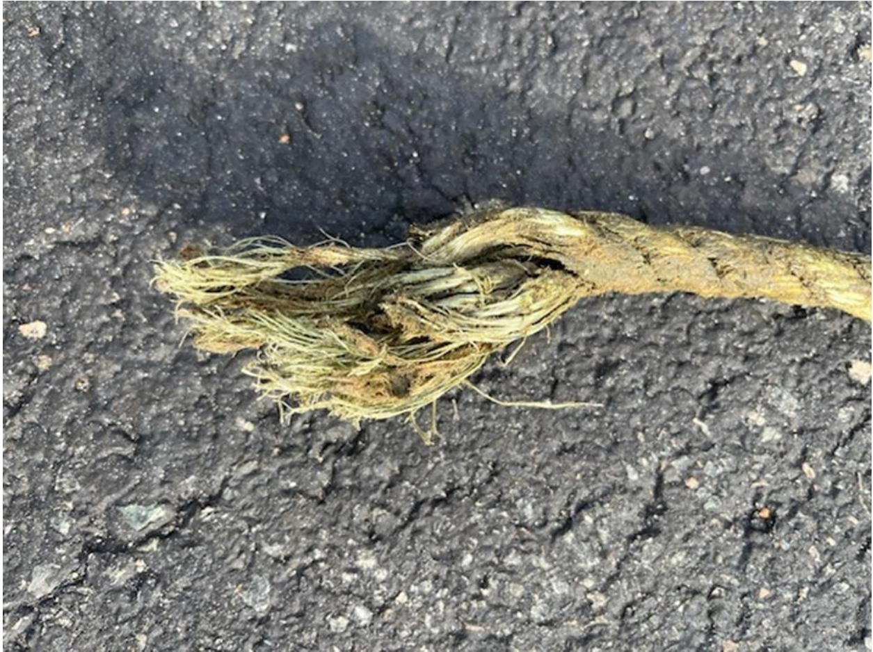
Fig. 15. Segment 1: Frayed end of 5/8 in. float rope, this was not one of the ends that was cut by the disentanglement efforts. This end would have led to the trap. Photo credit: Ed Trippel, DFO.
