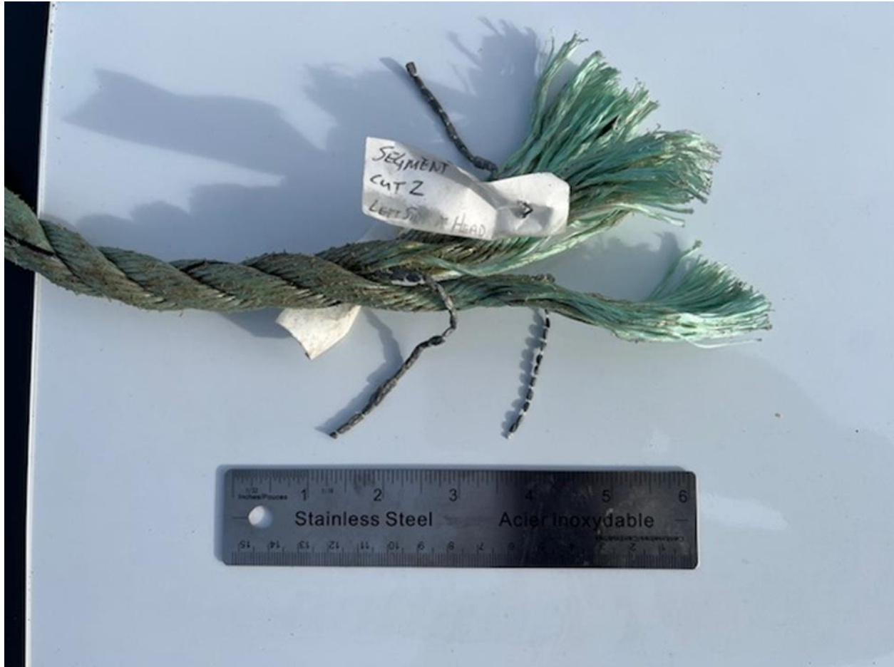
Fig. 7. Segment 2: A cut made by the disentanglement team of 5/8 in. sink rope. Beaded lead in each of the three strands are displayed. Photo credit: Ed Trippel, DFO.
