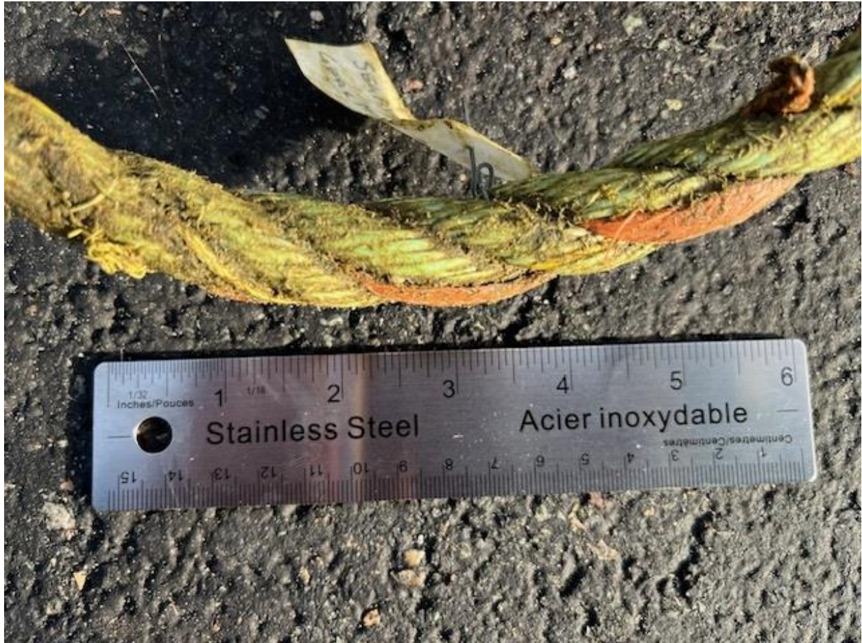
Fig. 12. Segment 1: Orange and yellow braided twines interlaced along a 7.9 inch (20 cm) section of 5/8 inch float rope. Twine sizes were 4 mm (orange) and 2.5 mm (yellow). Photo credit: Ed Trippel, DFO.
