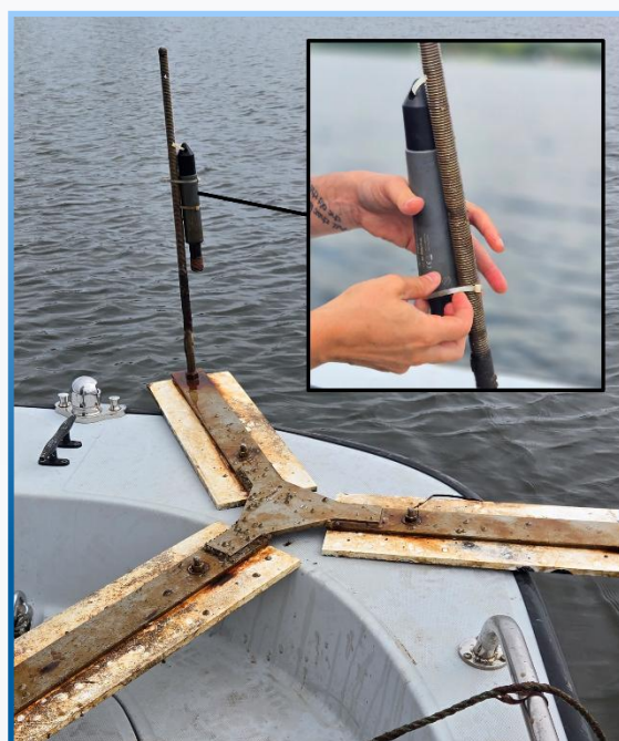
FG Figure 2: Dissolved oxygen logger attached to a rigid rebar post on a tripod foot, to keep the equipment standing vertically in the water column, and from sinking into the sediment. Photo credit: J. Walker, DFO.
