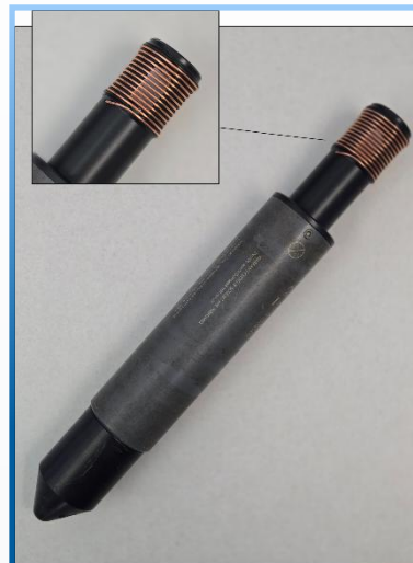
FG Figure 4: Copper wire guard on dissolved oxygen logger to reduce biofouling. Picture credit: J. Walker, DFO.
