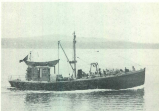
Figure 3. M/V "J. J. Cowie" used for drift-net fishing experiments in 1951 and 1952. Length overall 65 feet; Beam 15.3 feet; Gross tonnage 48.76; 100 h.p. Diesel engine.
