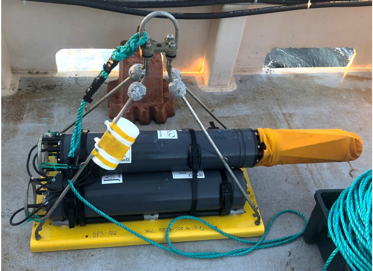
Figure 27. An AMAR autonomous acoustic recorder mooring prior to deployment to the seafloor.
