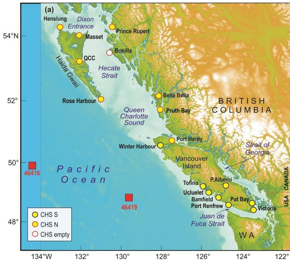
Figure 8. Map of British Columbia showing the locations of the Canadian Hydrographic Service (CHS) coastal tide gauges (indicated by circles) and open-ocean DART stations (indicated by red squares). Yellow circles with blue contours (CHS S) are CHS stations of the southern group of tide gauges that recorded the 2021 South Sandwich tsunami, the yellow circles with red contours (CHS N) are the same but for CHS tide gauges from the northern group; the white circle with the red contour (CHS empty) indicates the Bonilla station that did not record this tsunami.
