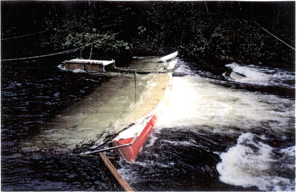
Photo 5. Kwinageese fence and video box at high water.
