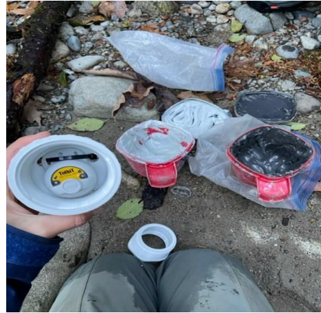
Figure 13: A HOBO Tidbit temperature logger secured inside a PVC end-cap
