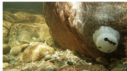
Figure 12: A PVC end-cap housing a HOBO Tidbit temperature data logger, which has been epoxied to a large boulder.
