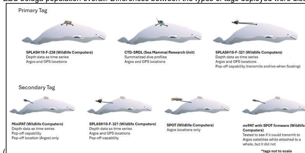
Figure 1). Harpoon-deployed tags have lower retention time than back-mounted tags. Back-mounted tags have longer retention times and will sink when released from a whale.
