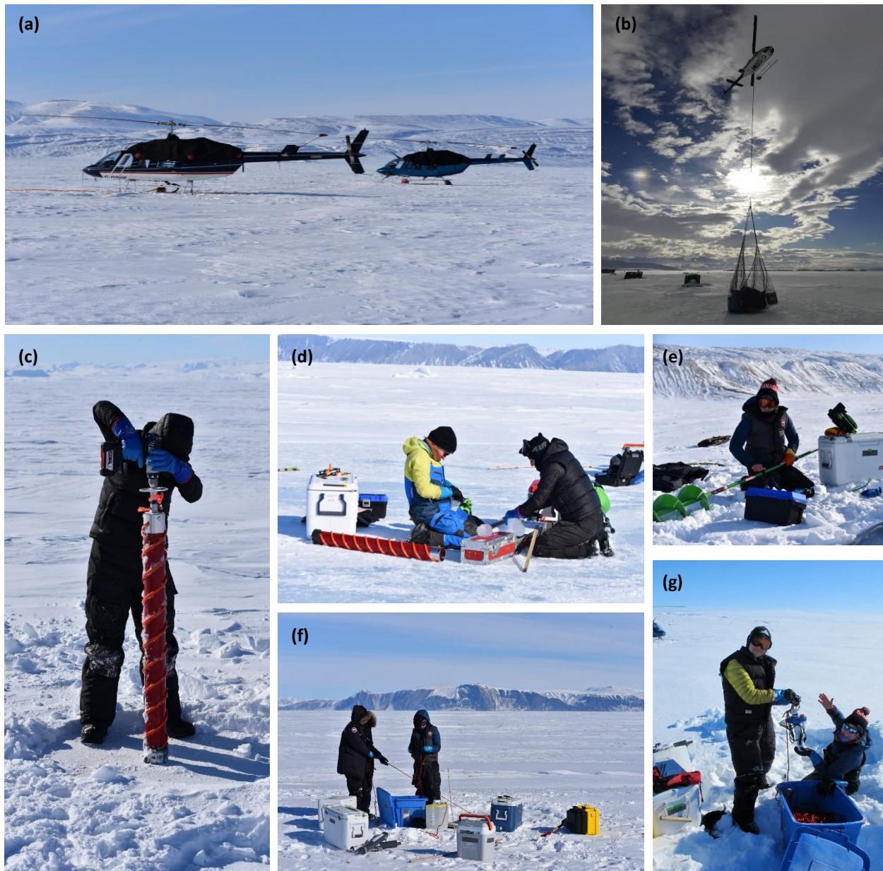
Figure 3. Overview of sampling activities including (a) Bell 206L helicopters used to transport field equipment and participants to and from stations, (b) helicopter sling operation to transport equipment, (c) sea ice sampling using a core barrel, (d) field participants cutting and bagging ice samples, (e) preparation of electric ice auger used to auger holes for water sampling, (f) recording of a CTD profile through a drilled ice hole, (g) field participants holding light and fluorescence sensor before deploying through a drilled ice hole (Source: ArcticCORE field team, 2024).
