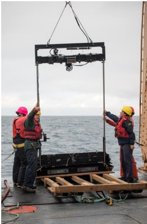
Figure 11. Recovering the MOCNESS plankton sampling net off the CCGS Tully. Photo credit: Jackson Chu
