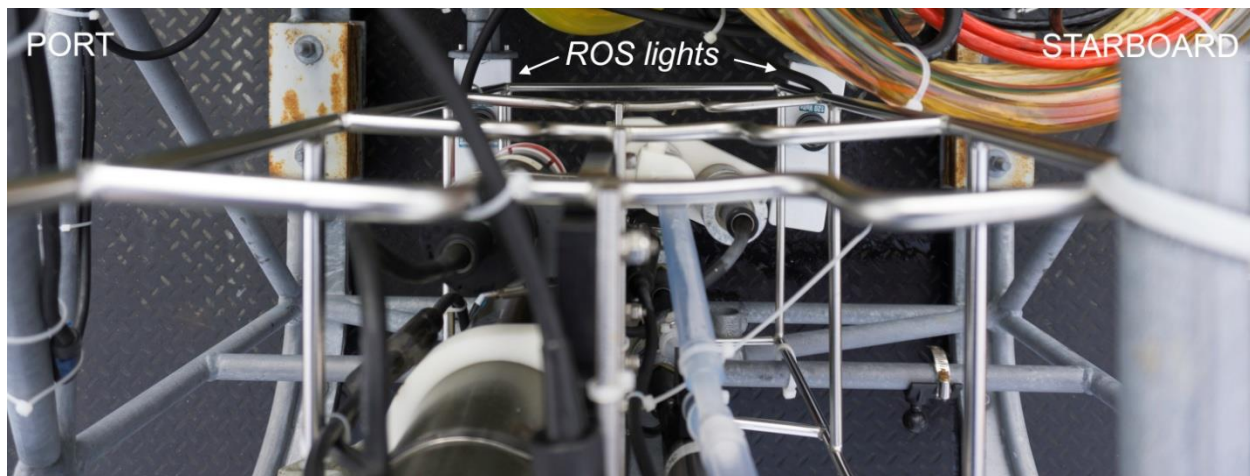
Figure A. 6. ROS light positions. Top-down view from above the CTD cage facing front of sled. Photo credit: Jackson Chu.
