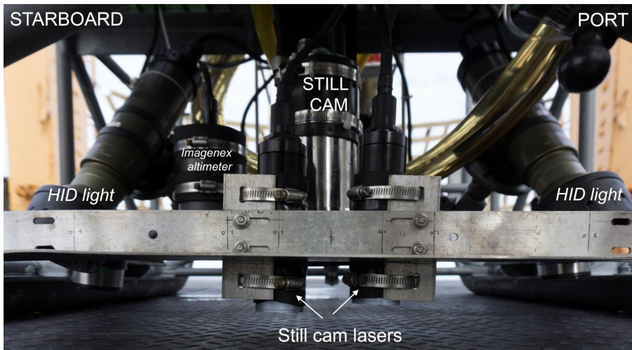
Figure A. 5. Stillcam laser mounting location at mid-section of sled. Facing rear of sled. Relative positions of scaling lasers for Stillcam for all dives B022-B032. Photo credit: Jackson Chu.
