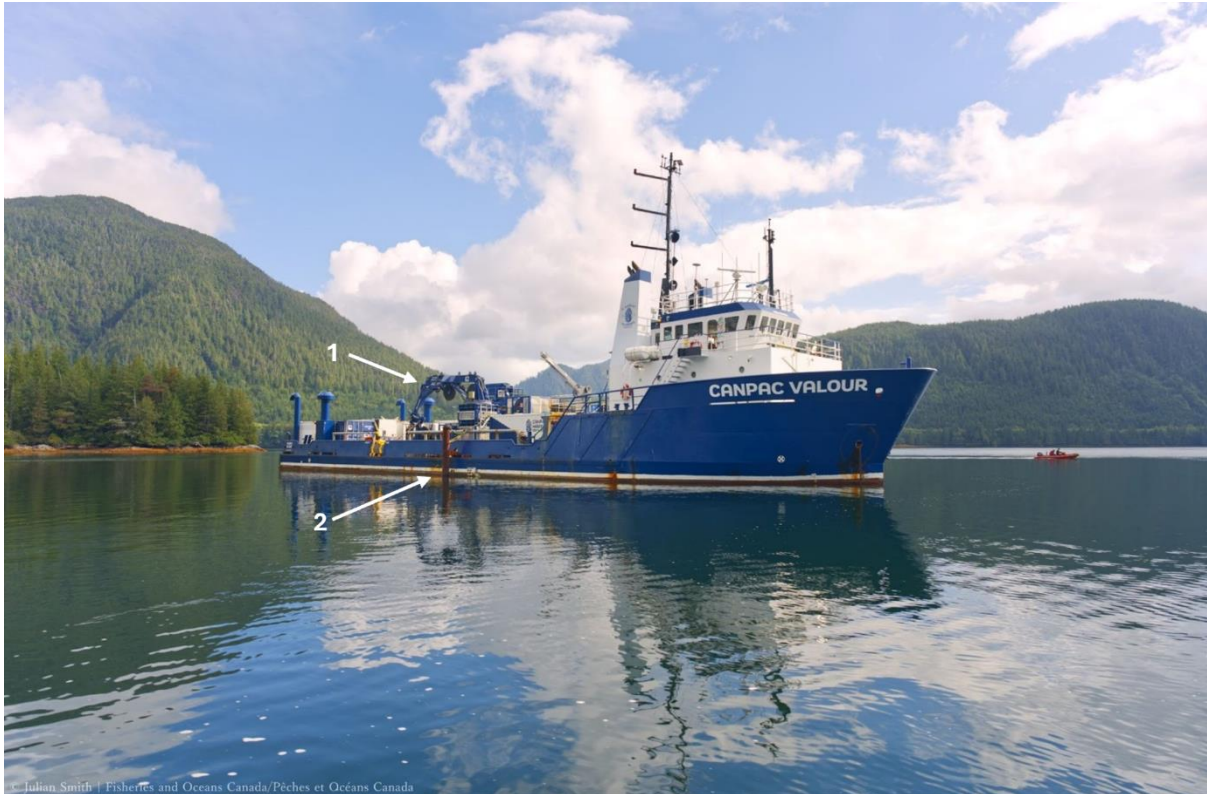
Figure 3. The motor vessel CanPac Valour at anchor. Labelled are 1 - The multibeam pole and 2 - the LARS crane as seen on the starboard side mid-ship. Image credits: Julian Smith, DFO
