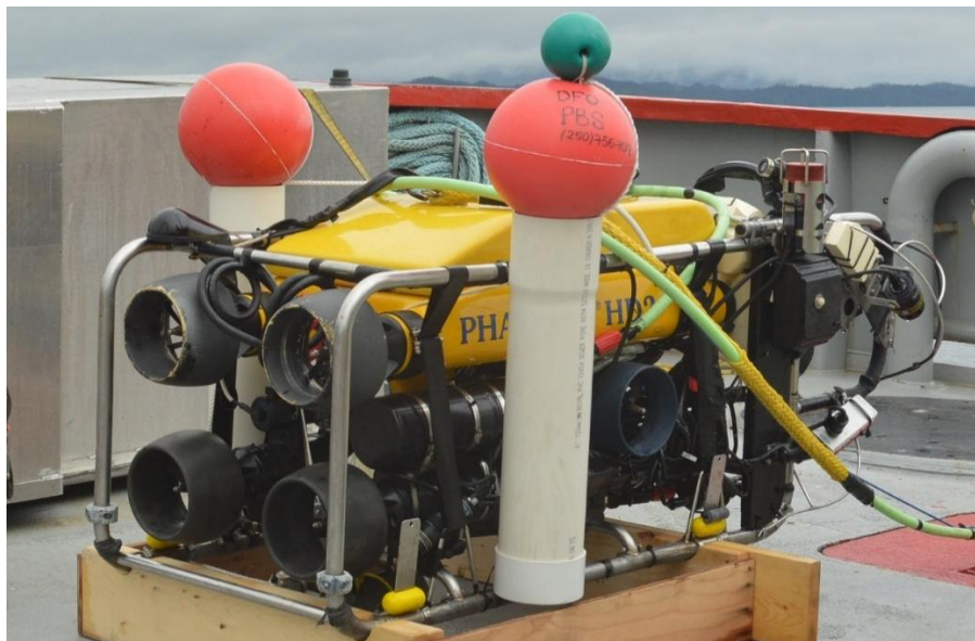
Figure 2: Phantom ROV on the aft deck of the CCGS Vector. Acoustic recorders for deployment were mounted inside the PCV pipes on either side of the ROV.
