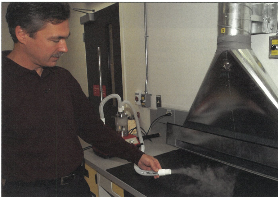
CCI conservation scientist Paul Marcon observes the airflow into a slot hood.
