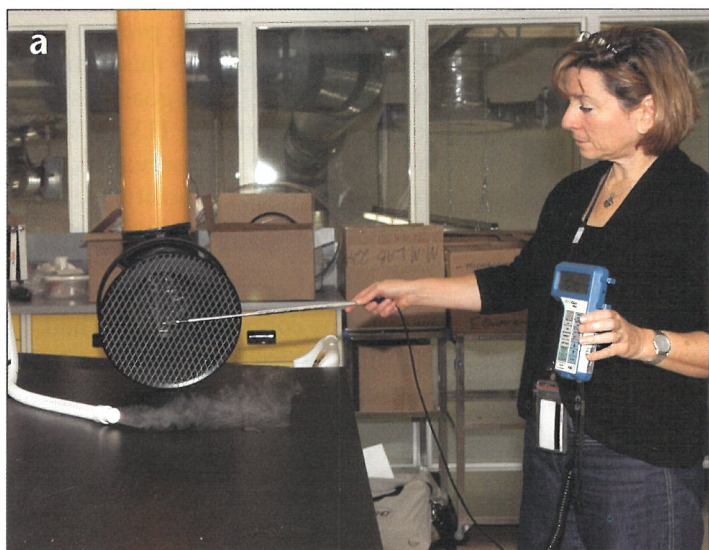
Source capture devices in action. (a) CCI conservation scientist Jane Sirois measures the airflow in a flexible arm. (b) CCI conservation intern Amanda Salmon applies varnish to a sample board while monitors measure the effectiveness of this bench-mounted slot hood in capturing the fumes released.
