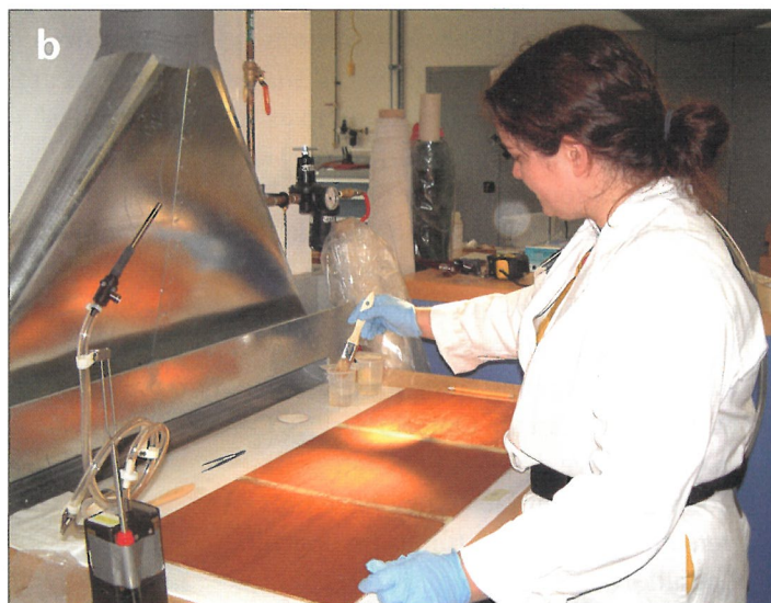
Source capture devices in action. (a) CCI conservation scientist Jane Sirois measures the airflow in a flexible arm. (b) CCI conservation intern Amanda Salmon applies varnish to a sample board while monitors measure the effectiveness of this bench-mounted slot hood in capturing the fumes released.
