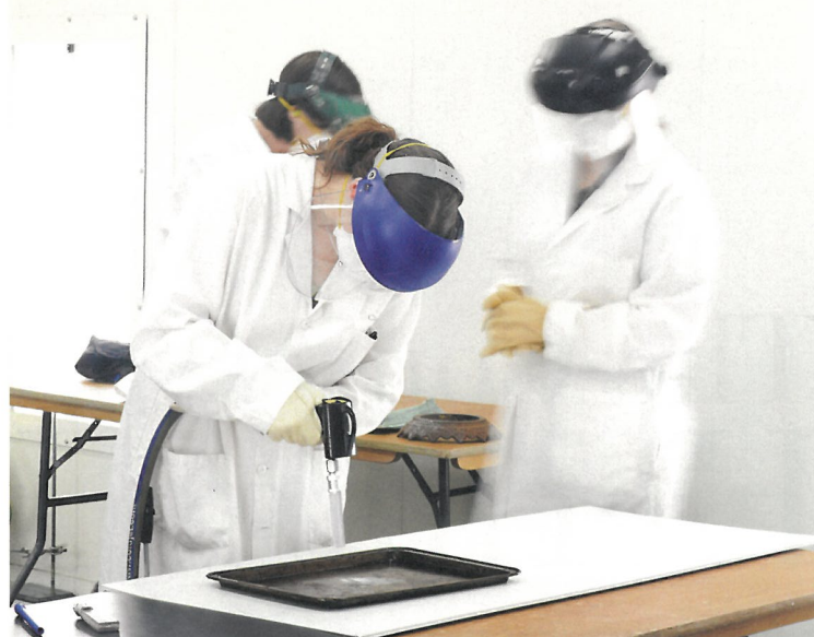
▲ Interns and emerging conservators were part of the team testing the performance of a micro-blasting CO 2 (dry ice) machine.
