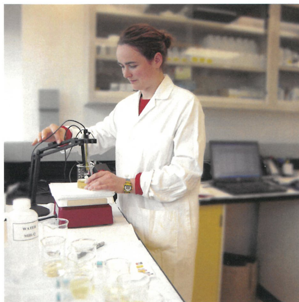
▲ CCI archaeology and objects intern Ute Werner measures the concentration of chloride ions.
