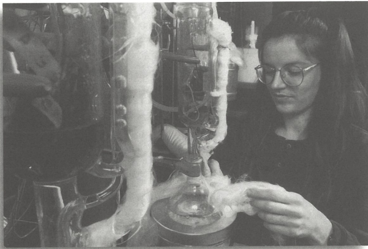
Hot-washing composite artifacts in the Soxhlet system.
