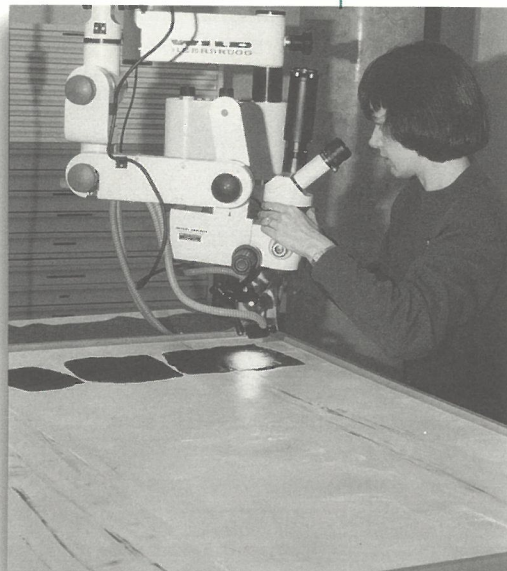
Taking a paint sample from a Borduas painting.
