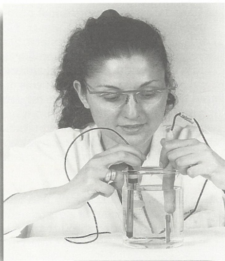
Measuring the corrosion potential of iron.
