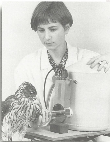
Using a portable x-ray spectrometer to identify toxic compounds in a specimen.
