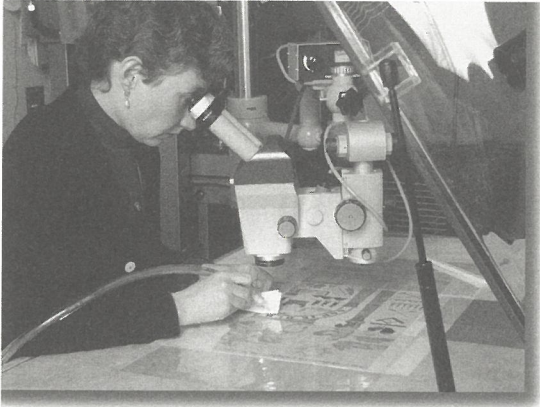
Consolidating areas of a fragile watercolour using an ultrasonic mister and a paper suction table.
