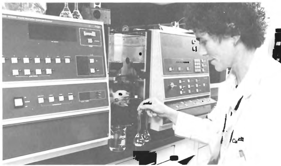
The author using atomic absorption spectrophotometry to determine trace element profiles in artifact studies.
