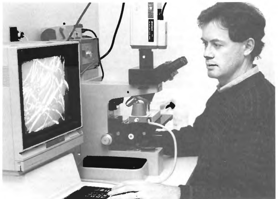
Greg Young examining collagen fibres with microscope thermal microscopy stage and video monitor.
