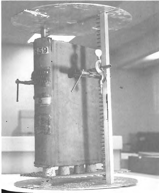
A ledger with red-rot about to undergo a test coating with Parylene.
