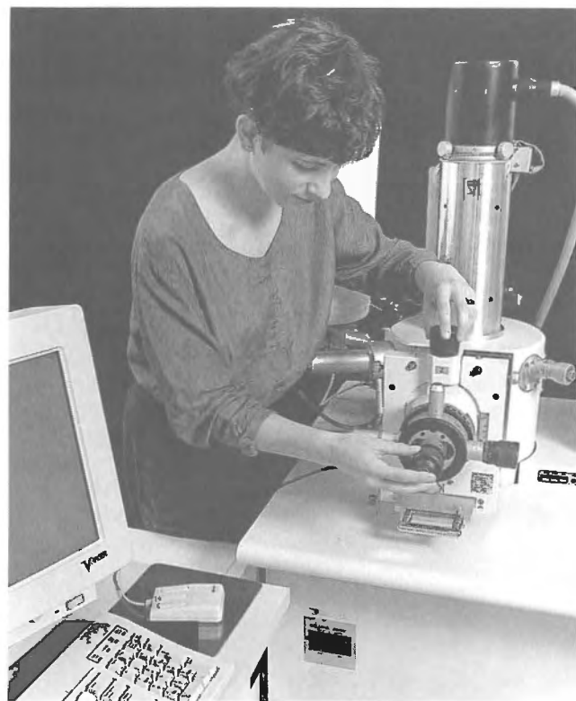
Figure 1. Kate Helwig inserts a specimen into the sample chamber of the scanning electron microscope for x-ray microanalysis.
