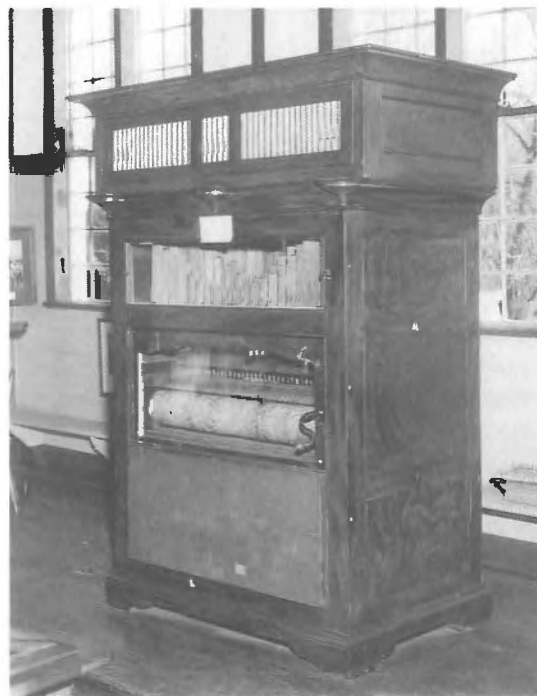
Figure 2. The barrel organ supplied by Richard Coates. The barrel lies horizontally below the pipes and is turned by a crank-and-worm gear. The bellows is in the casework below the barrel, although at the time this picture was taken an electric blower had been installed.
