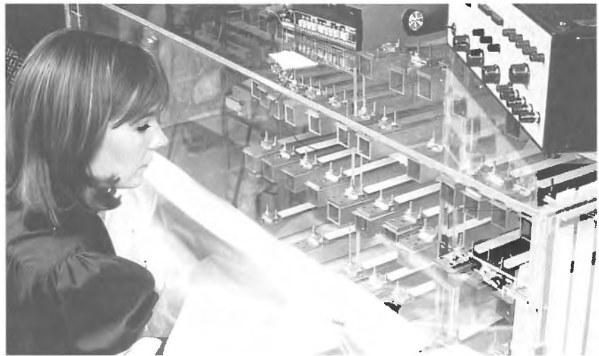
Testing the effects of changing RH on the behaviour of model canvas paintings and lining materials.
