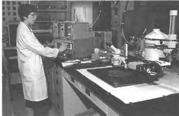
Figure 1. A painting is examined with the x-ray energy spectrometer.
