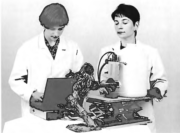
Figure 3. A natural history specimen is analyzed in the portable spectrometer.
