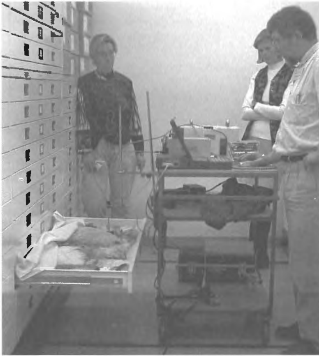
Figure 1. Scott Williams uses the portable IR Spectrometer to analyze fans in storage drawers at the ROM while being assisted by Shannon Elliot and Jackie Spafford of the ROM.
