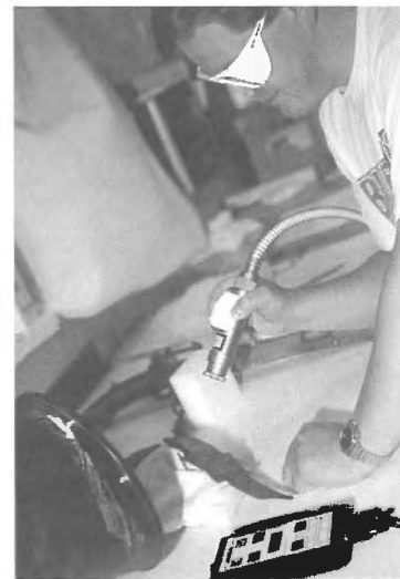
Removing surface dirt from leather. The unit in the foreground controls the power and other cleaning parameters.
