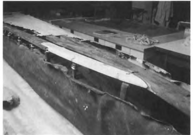
Replacement portion of the missing bilge stringer. The kayak is upside down and the original canvas has been folded back, revealing the remains of the original sealskin.
