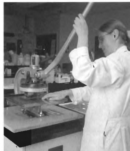
Irene Karsten cuts samples of adhesive films before measuring their tensile properties.
