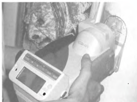
Measurement of original paint, Ontario Legislative Building, Queen's Park, Toronto.
