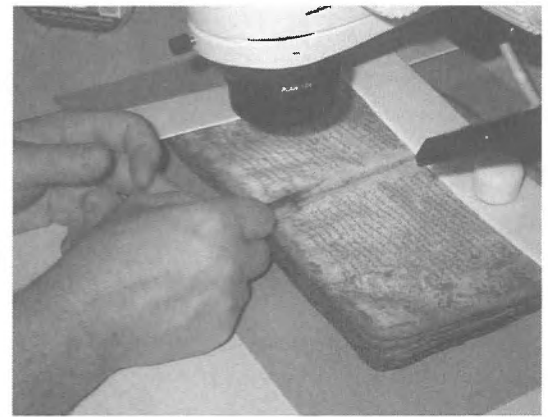
While viewing the palimpsest through a stereomicroscope, Scott takes a sample of adhesive using a scalpel.
