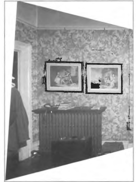
The rectified image. The wall now appears head on instead of at an angle.
