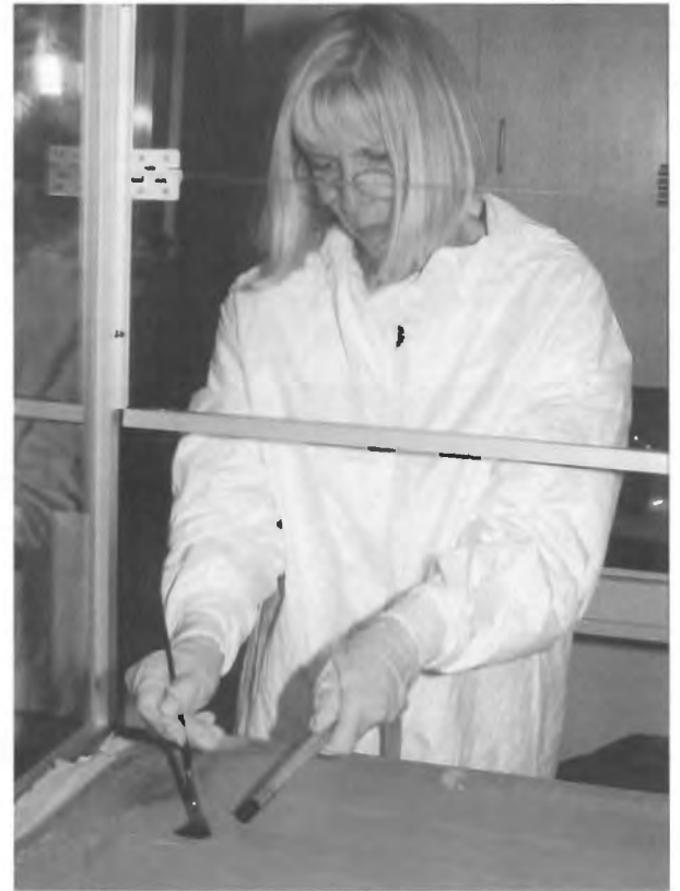
Conservator working at a class 1 biological safety enclosure. Note that the vacuum cleaner nozzle is secured inside the hood. This helps ensure the nozzle does not accidentally touch the artifact and that the contaminated nozzle remains in the enclosure.
