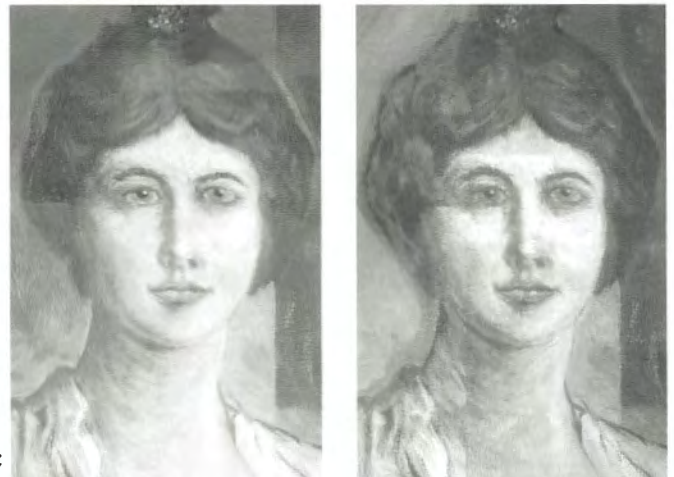
An image captured using normal digital photography (left) as compared with one captured using ultraviolet fluorescence technique (right).
