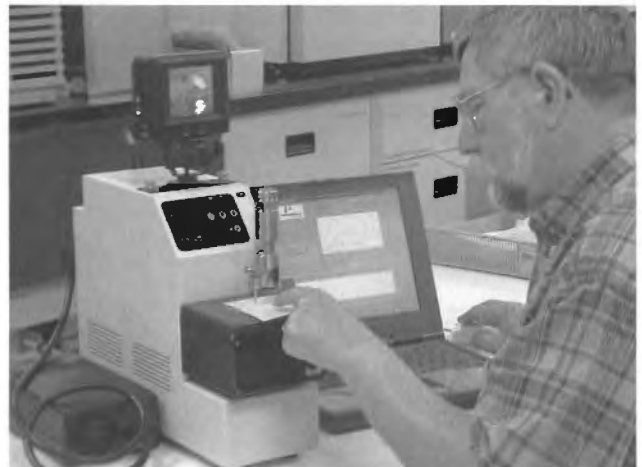
Figure 4. The TravelIR (Sensir Technologies) ATR IR spectrometer in operation. The sample or object to be analysed is placed on the crystal under the presser bar indicated by the pointing finger.
