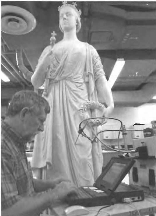
Figure 3. By observing the IR spectra after each stage of treatment, Scott is able to monitor the effects of cleaning solutions on the marble of this statue of Queen Victoria.
