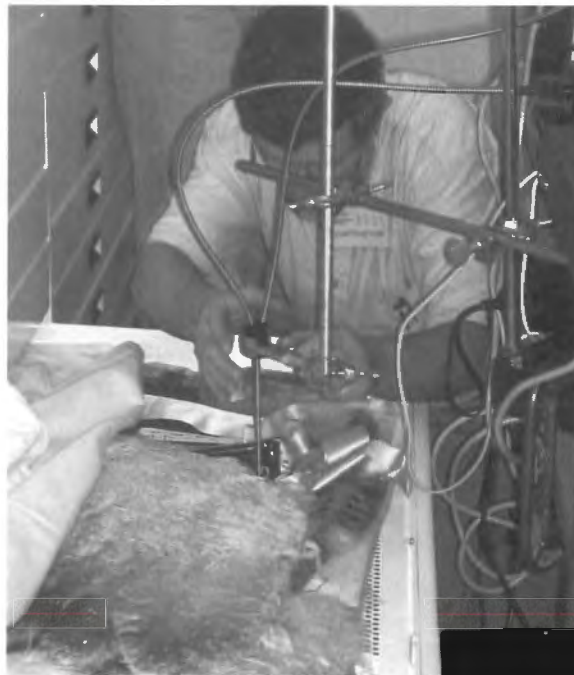
Figure 2. The FOP spectrometer can be brought directly to fragile objects such as these feather fans. This allows fragile objects to be analysed without ever having to be handled, touched, or sampled.
